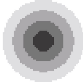
Figure 4 Partitioning of the DFT domain. Different grey scales indicate different regions. The image centre at frequency 0
